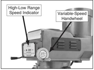
**Figure 33.** Model G0748 variable-speed controls.
